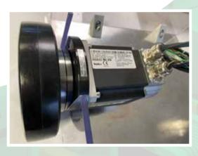
Mounted from inside the AGV, the bolts go through the motor mounting plate from the rear and attach to the inside of the AGV body. Take care in leaving enough clearance between the AGV motor wheel and the AGV body.
